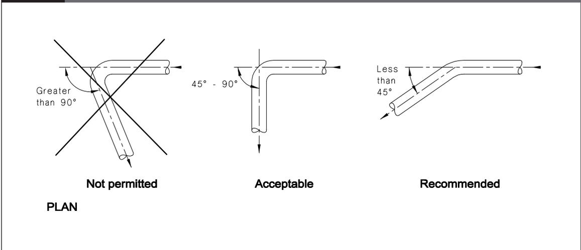
**Figure 5: Junction of Drains**
