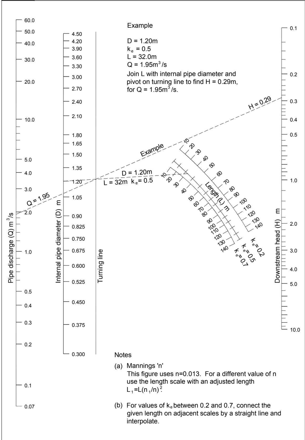
**Figure 11: Downstream Head for Box Culverts**
