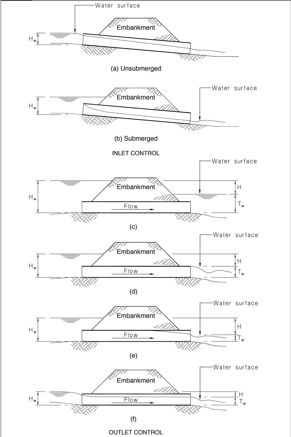
**Figure 6: Headwater Depth for Circular Pipes**
