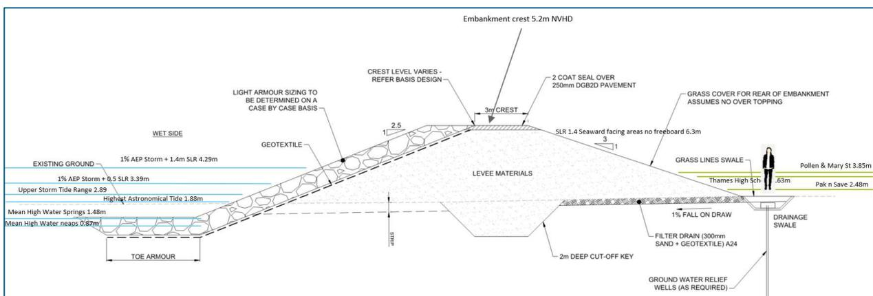
**Figure 36:** Thames possible coastal defence crest levels compared to oceanic and landside elevations
