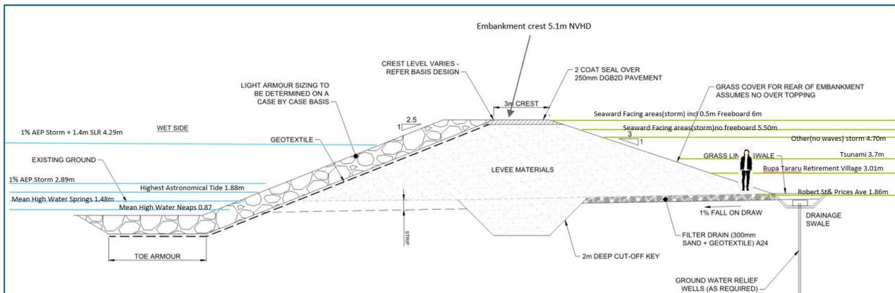
Figure 27: Tararu possible defence crest levels compared to oceanic and landside elevations
