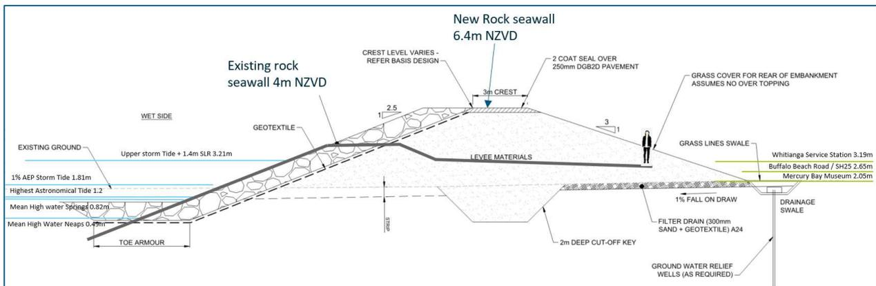
Figure 14: Whitianga possible coastal defence crest levels compared to oceanic and landside elevations
