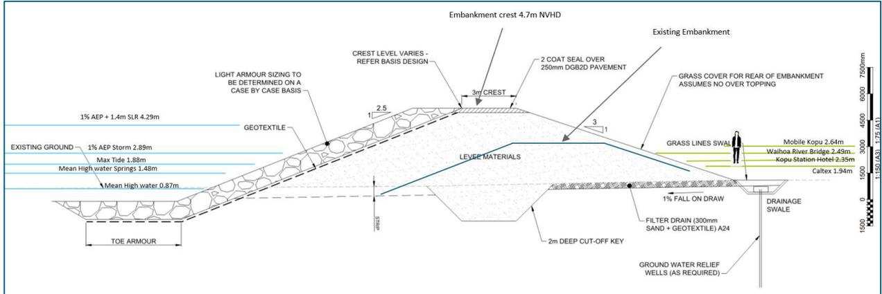
Figure 41: Possible future coastal defence crest level for Kopu compared to oceanic and landside elevations
