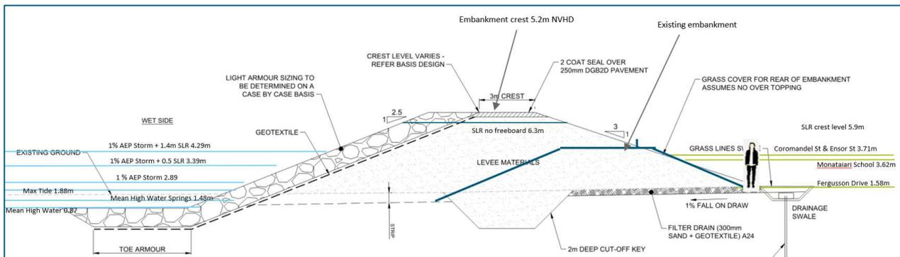
Figure 32 Moanataiari possible defence crest levels compared to oceanic and landside elevations
