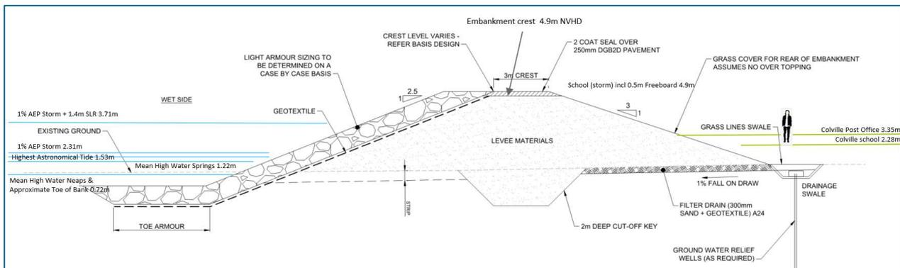
**Figure 20:** Colville possible defence crest levels compared to oceanic and landside elevations
