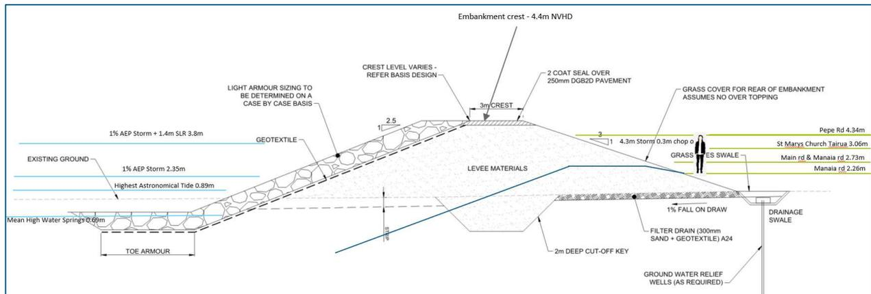
Figure 12: Tairua possible defence crest levels compared to oceanic and landside elevations
