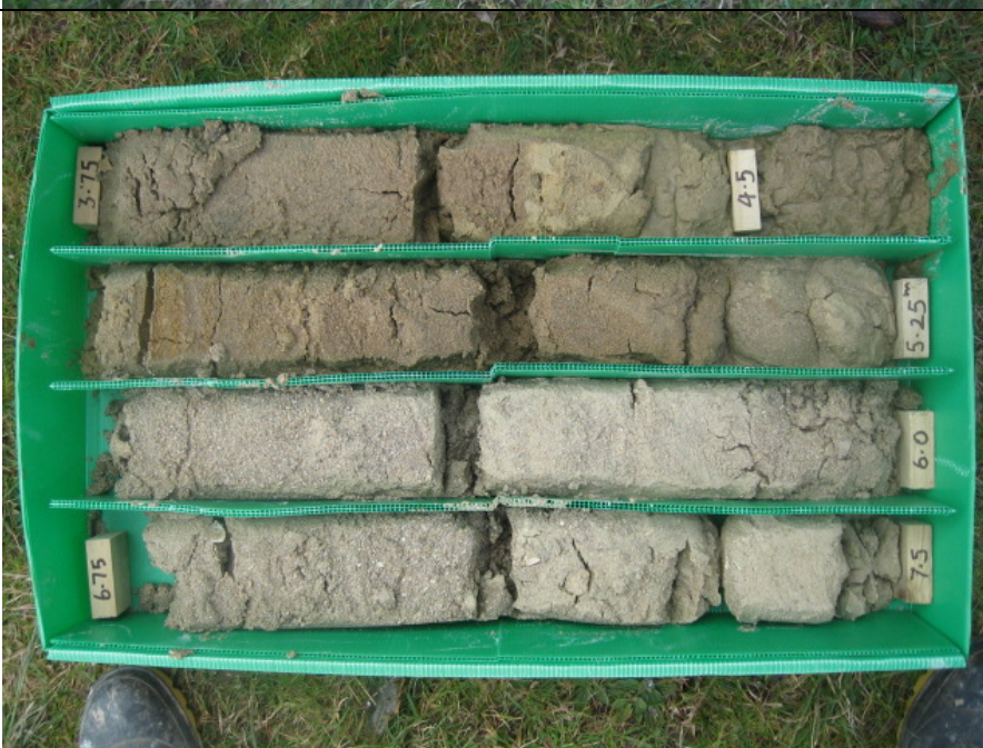
Photo 6: BH 02 PQ core from 3.75m to 7.5m depth. No core recovery from 7.5m to 8.2m
