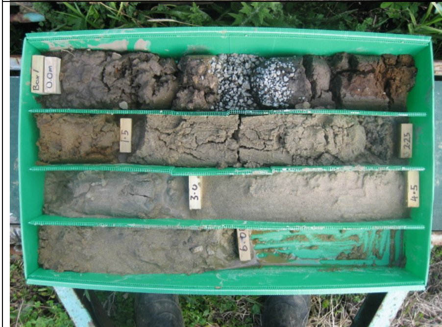
Photo 2: BH 02 PQ core from 0m to 6m depth
