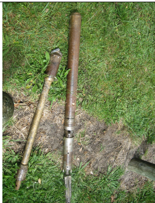
Cutter bit and sampling tube fit inside stem
