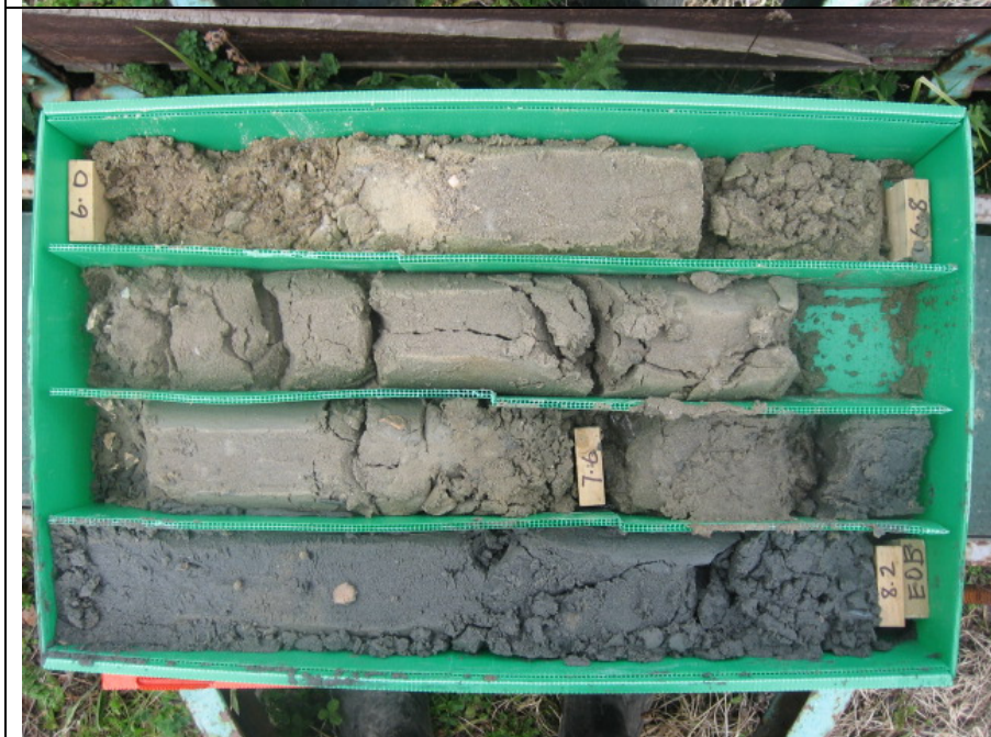
Photo 3: BH 02 PQ core from 6m to 8.2m depth
