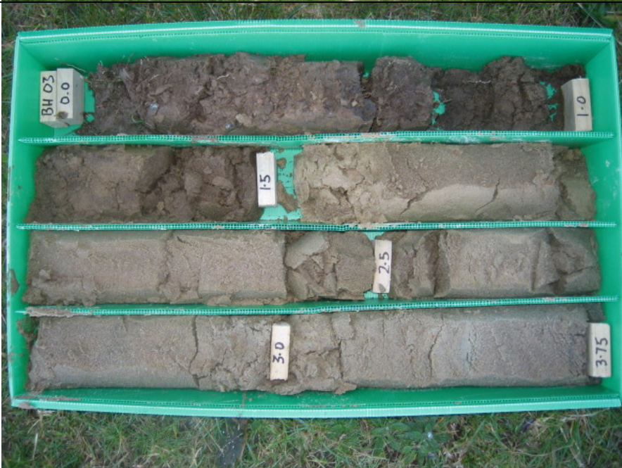
Photo 5: BH 03 PQ core from 0m to 3.75m depth
