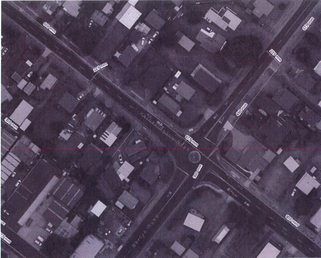
Figure 3-12 Reduction pipe diameter on Hetherington Road
