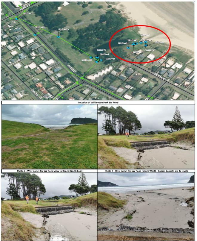
Photo 6 - Weir outlet for SW Pond view to Pond - Gabian baskets are 4x levels
